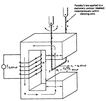
Fcc 6-22 It is impossible to design a commutatorless dc machine. Although the speed voltage alone can have a dc average, it will be canceled by the transformer electromotive force due to the time rate of change of magnetic flux through the loop. The total terminal voltage will always have a zero time average.
