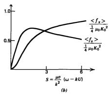
Figure 6-29 (a) A traveling wave of surface current induces currents in a conductor that is moving at a velocity U different from the wave speed  $\omega/k$ . (b) The resulting forces can levitate and propel the conductor as a function of the slip S, which measures the difference in speeds of the conductor and traveling wave.
