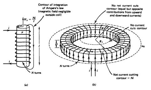
Figure 6-10 Inductances. (a) Solenoidal coil; (b) toroidal coil.
