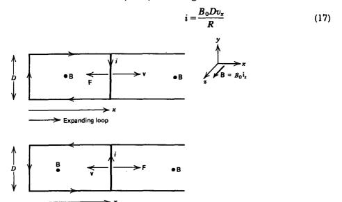
Figure 6-5 If a conductor moves perpendicular to a magnetic field a current is induced in the direction to cause the Lorentz force to be opposite to the motion. The total flux through the closed loop, due to both the imposed field and the self-field generated by the induced current, tries to remain constant.
