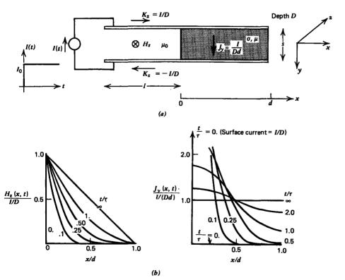
Figure 6-26 (a) A current source is instantaneously turned on at t=0. The resulting magnetic field within the Ohmic conductor remains continuous and is thus zero at t=0 requiring a surface current at x=0. (b) For later times the magnetic field and current diffuse into the conductor with longest time constant  $\tau = \sigma \mu d^2/\pi^2$  towards a steady state of uniform current with a linear magnetic field.
