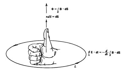
Figure 6-2 Faraday's law states that the line integral of the electric field around a closed loop equals the time rate of change of magnetic flux through the loop. The positive convention for flux is determined by the right-hand rule of curling the fingers on the right hand in the direction of traversal around the loop. The thumb then points in the direction of positive magnetic flux.
