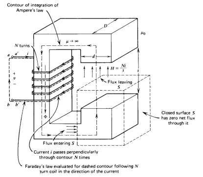
Figure 6-8 The magnetic field is zero within an infinitely permeable magnetic core and is constant in the air gap if we neglect fringing. The flux through the air gap is constant at every cross section of the magnetic circuit and links the N turn coil N times.
