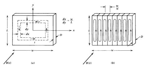
Figure 6-6 (a) A time varying magnetic field through a conductor induces eddy currents that cause Ohmic heating. (b) If the conductor is laminated so that the induced currents are confined to thin strips, the dissipated power decreases.
