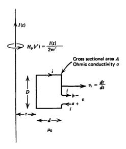
Figure 6-4 A rectangular loop near a time varying line current. When the terminals are short circuited the electromotive force induces a current due to the time varying mutual flux and/or because of the motion of the circuit through the imposed nonuniform magnetic field of the line current. If the loop terminals are open circuited there is no induced current but a voltage develops.
