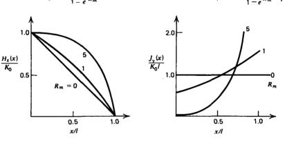
Figure 6-28 (a) A conducting material moving through a magnetic field tends to pull the magnetic field and current density with it. (b) The magnetic field and current density are greatly disturbed by the flow when the magnetic Reynolds number is large,  $R_m = \sigma \mu U l \gg 1$ .
