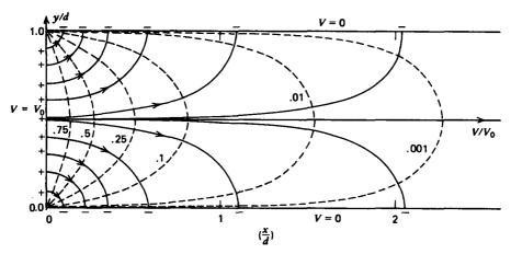
Figure 4-5 An open conducting box of infinite extent in the x and z directions and of finite width d in the y direction, has zero potential on all surfaces except the closed end at x = 0, where  $V = V_0$ .
