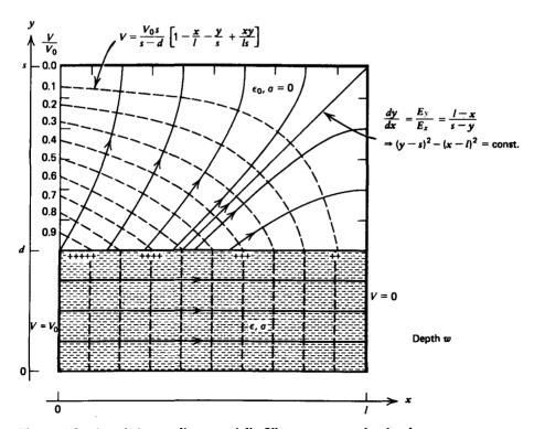
Figure 4-2 A resistive medium partially fills an open conducting box.
