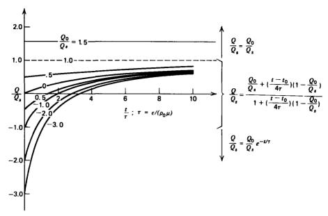
Figure 4-14 There are three regimes describing the charge build-up on the sphere. It takes many time constants  $[\tau = \varepsilon/(\rho_0 \mu)]$  for the charge to approach the saturation value  $Q_n$ , because as the sphere charges up the Coulombic repulsive force increases so that most of the charge goes around the sphere. If the sphere is externally charged to a value in excess of the saturation charge, it remains constant as all additional charge is completely repelled.
