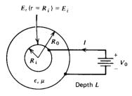
(a) The electric field at the emitter electrode is given as  $E_r(r = R_i) = E_i$ . If a current I flows, what are the steady-state electric field and space charge distributions?
