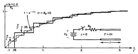
Figure 8-12 The open circuit voltage at z=l for a step voltage applied at t=0 through a source resistance R, for various values of  $T/\tau$ , which is the ratio of propagation time T=l/c to quasi-static charging time  $\tau=R$ , Cl. The dashed curve shows the exponential rise obtained by a circuit analysis assuming the open circuited transmission line is a capacitor.
