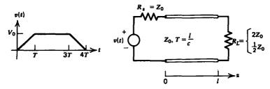
12. A step voltage is applied to a loaded transmission line with  $R_L = 2Z_0$  through a matching source resistor.
