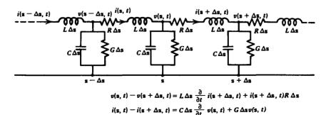
Figure 8-5 Distributed circuit model of a transmission line including small series and shunt resistive losses.
