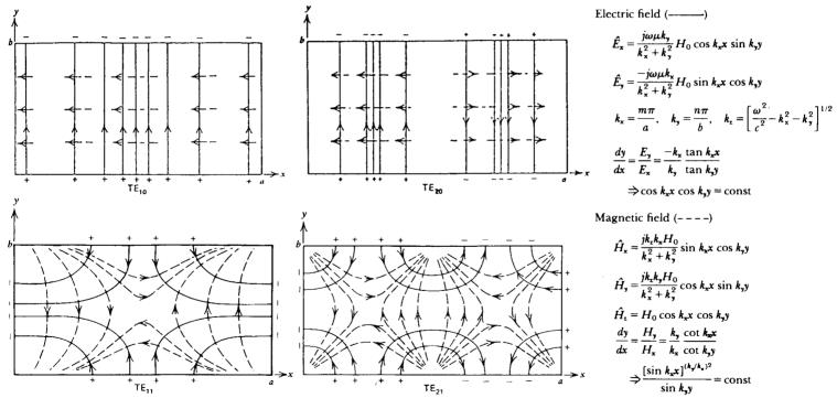
Figure 8-29 (a) The transverse electric and magnetic field lines for various TE modes. The magnetic field is purely z directed where the field lines converge. The TE<sub>10</sub> mode is called the dominant mode since it has the lowest cut-off frequency. (b) Surface current lines for the TE<sub>10</sub> mode.
