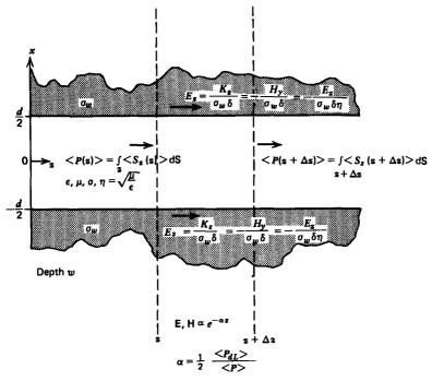
Figure 8-16 A transmission line with lossy walls and dielectric results in waves that decay as they propagate. The spatial decay rate  $\alpha$  of the fields is approximately proportional to the ratio of time average dissipated power per unit length  $< P_{dL} >$  to the total time average electromagnetic power flow < P > down the line.
