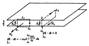
Figure 8-2 The potential difference measured between any two arbitrary points at different positions  $z_1$  and  $z_2$  on the transmission line is not unique—the line integral  $L_1$  of the electric field is nonzero since the contour has magnetic flux passing through it. If the contour  $L_2$  lies within a plane of constant z such as at  $z_3$ , no magnetic flux passes through it so that the voltage difference between the two electrodes at the same value of z is unique.
