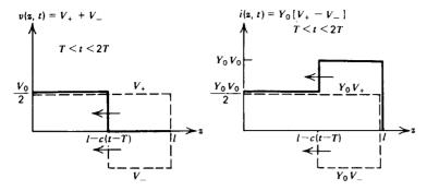
Short circuited line,  $R_L = 0$ ,  $(v(z, t \ge 2T) = 0$ ,  $i(z, t \ge 2T) = Y_0 V_0)$
