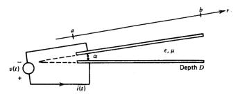
4. A parallel plate transmission line is filled with a conducting plasma with constitutive law
