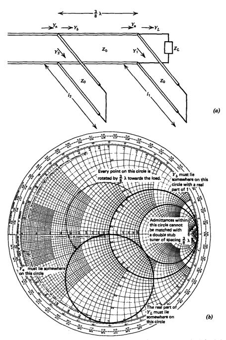
Figure 8-25 (a) A double stub tuner of fixed spacing cannot match all loads but is useful because additional elements can only be placed at transmission line terminations and not at any general position along a line as required for a single-stub tuner. (b) Smith chart construction. If the stubs are  $\frac{3}{8}\lambda$  apart, normalized load admittances whose real part exceeds 2 cannot be matched.
