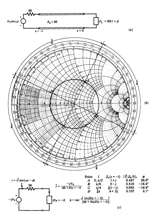
Figure 8-20 (a) The load impedance at z = 0 reflected back to the source is found using the (b) Smith chart for various line lengths. Once this impedance is known the source current is found by solving the simple series circuit in (c).
