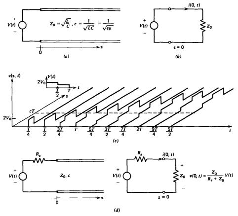
Figure 8-6 (a) A semi-infinite transmission line excited by a voltage source at z = 0. (b) To the source, the transmission line looks like a resistor  $Z_0$  equal to the characteristic impedance. (c) The spatial distribution of the voltage v(z,t) at various times for a staircase pulse of V(t). (d) If the voltage source is applied to the transmission line through a series resistance  $R_n$  the voltage across the line at z = 0 is given by the voltage divider relation.
