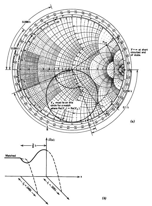
Figure 8-26 (a) The Smith chart construction for a double-stub tuner of  $\frac{3}{8}\lambda$  spacing with  $Z_{nL} = 1 + j$ . (b) The voltage standing wave pattern.
