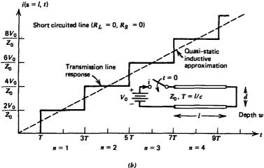
Figure 8-11 The (a) open circuit voltage and (b) short circuit current at the z = l end of the transmission line for  $R_s = 0$ . No dc steady state is reached because the system is lossless. If the short circuited transmission line is modeled as an inductor in the quasi-static limit, a step voltage input results in a linearly increasing current (shown dashed). The exact transmission line response is the solid staircase waveform.
