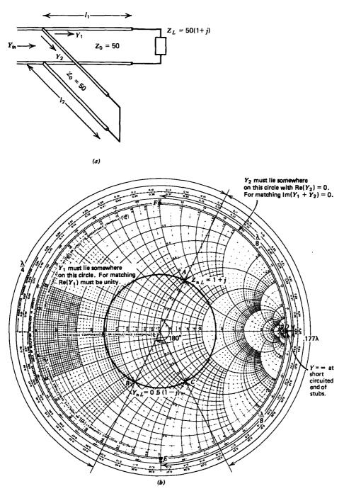
Figure 8-24 (a) A single stub tuner consisting of a variable length short circuited line  $l_2$  can match any load to the line by putting the stub at the appropriate distance  $l_1$  from the load. (b) Smith chart construction. (c) Voltage standing wave pattern.
