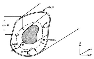
Figure 8-4 A general transmission line has two perfect conductors whose cross-sectional area does not change in the direction along its z axis, but whose shape in the transverse xy plane is arbitrary. The electric and magnetic fields are perpendicular, lie in the transverse xy plane, and have the same dependence on x and y as if the fields were static.
