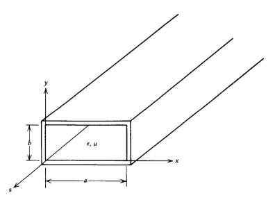
Figure 8-27 A lossless waveguide with rectangular cross section.
