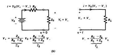
Figure 8-8 (a) A dc voltage  $V_0$  is switched onto a resistively loaded transmission line through a source resistance  $R_z$  (b) The equivalent circuits at z = 0 and z = l allow us to calculate the reflected voltage wave amplitudes in terms of the incident waves.
