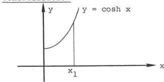
$$s = \int_{0}^{x_{1}} \sqrt{1 + \left(\frac{dy}{dx}\right)^{2}} dx = \int_{0}^{x_{1}} \cosh x dx = \sinh x_{1}$$
