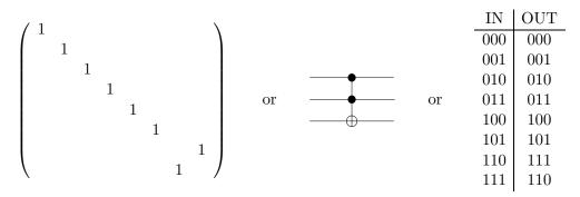
This gate is universal: with ancillary input zeros, it can be used to compute any function.
