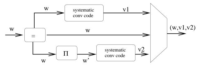
Figure 15.1: Turbo Encoder. The "=" node can be viewed as a repetition code that sends its input 3 ways. The  $\Pi$  node represents the permutation. Note that the block length must be fixed so that  $\Pi$  can be fixed. The object on the right just interleaves the three streams. This is Figure 3.8 in Fan.
