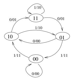
Figure 14.3: The finite automaton for the encoder in Figure 2. Each state is labeled with the Each transition has a label of the form  $w/v_1v_2$ , where w represents the input bit and  $v_1$  and  $v_2$  represent the two output bits. In this case, we always have  $w = v_1$ .
