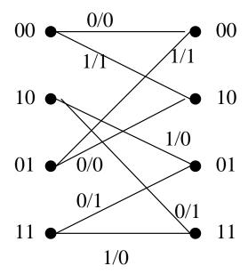
Figure 14.5: A trellis section. The nodes represent the states, and the transisions are labeled by input/other output.
