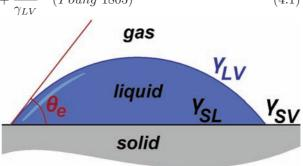
Figure 4.1: Three interfaces meet at the contact line.
