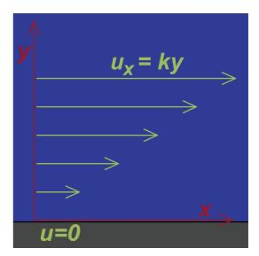
Figure 4.5: Shear flow above a rigid lower boundary.
