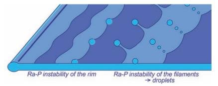
Figure 12.6: The typical evolution of a retracting sheet. As the rim retracts and engulfs fluid, it eventually becomes Rayleigh-Plateau unstable. Thus, it develops variations in radius along its length, and the retreating rim becomes scalloped. Filaments are eventually left by the retracting rim, and pinch off through a Rayleigh-Plateau instability, the result being droplets.
