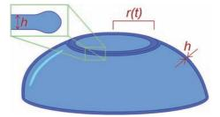
(2.15) Figure 12.3: Rupture of a soap film of thickness h.
