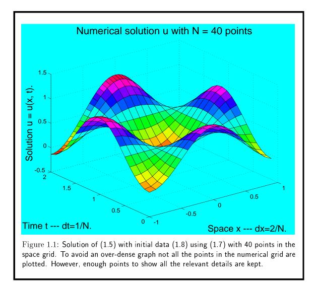
Figure 1.1 shows the result of this calculation using N = 40. Note that the periodicity in time fails to hold. In fact, after one time period the numerical method appears to have **amplified** the initial
