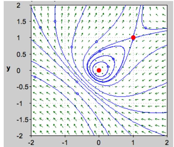
This is *structurally stable*  $\Rightarrow$  the nonlinear system has a saddle at  $(1,1)$ .
