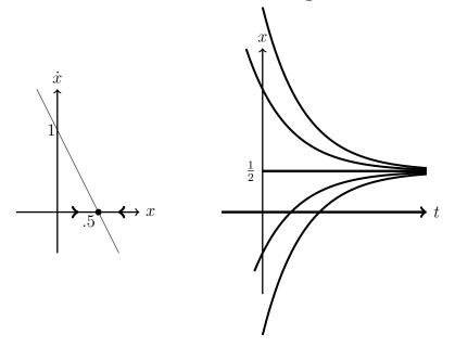
c) We use Euler's method.  $\frac{dx}{dt} = f(t, x) = 1 - 2x$  with  $t_0 = 0$  and  $x_0 = x(t_0) = x(0) = 0$  (given). We then have:
