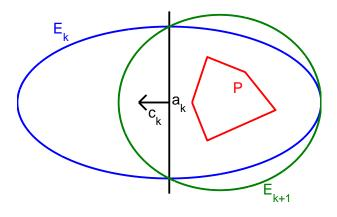
Figure 1: Diagram illustrating a single iteration of the ellipsoid algorithm.
