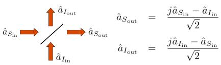
Output State from 50/50 Beam Splitter:
