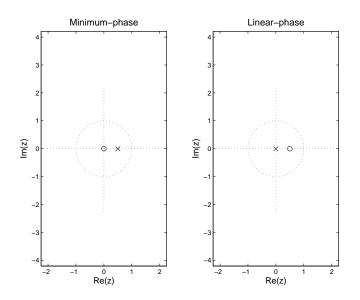
Combining these, the minimum-phase system and FIR linear-phase systems are as shown below.
