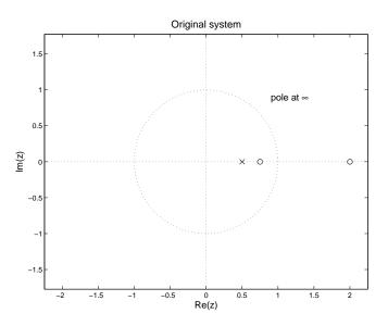
(a) One way to carry out the minimum-phase and all-pass decomposition is as follows. In the first stage, collect all zeros and poles that are inside the unit circle (zero at z = 3/4, pole
