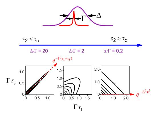
In the inhomogeneous limit, an echo ridge decaying as  $e^{-\Gamma t}$  extends along  $\tau_1 = \tau_3$ . It decays with the inhomogeneous distribution in the perpendicular direction. In the homogeneous limit, the response is symmetric in the two time variables. Fourier transformation allows these envelopes to be expressed as the lineshapes above. Here again  $\tau_2$  is a control variable to allow us to characterize  $C_{ee}(\tau)$  through the change in echo profile or lineshape.
