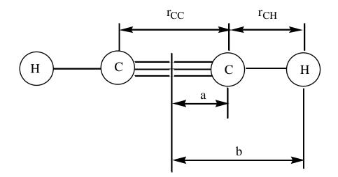
Solve for the moments of inertia of two of the isotopomers in terms of these distances and then solve these equations simultaneously. Report the bond lengths with errors and compare to literature values. Be careful with units; report your values and literature values in the same set of units. Compare the bond lengths to typical values for C-H and C=C bonds. Would you have been able to calculate the bond lengths if you had only taken the spectrum of one isotopomer?
