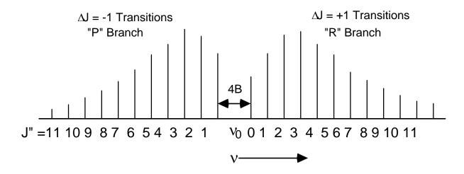
The intensity profile is the product of a linearly increasing function and an exponentially decreasing function. At large J the exponential decrease takes over, but at small J the
