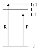
Traditionally, the upper state is denoted by single primes and the lower state by double primes, so the upper and lower state rotational energies are
