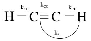
To a very crude approximation, the potential energy can be described by three force constants,  $k_{CH}$ ,  $k_{CC}$ , and  $k_{\delta}$ . If we define deviations from equilibrium bond lengths as  $x_A$  and  $x_B$  for the two C-H stretches and y for the C=C stretch, and deviations from the linear bond angles as  $\delta_A$  and  $\delta_B$  then the potential energy of the molecule would be modeled as
