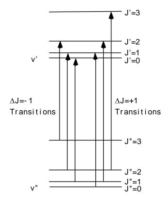
Each allowed transition results in an absorption line in the IR spectrum. The  $\Delta J =$  -1 and  $\Delta J =$  +1 transitions are referred to as P- and R-branch lines respectively. The energy difference between any two adjacent lines in the P and R branches is given by 2B<sub>e</sub> (in wavenumbers). Thus, the spectrum has the following structure:
