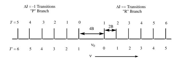
The vibrational energy can be determined immediately as the midpoint of the first two transitions in the P and R branches. The rotational constant can be determined simply from the spacing between the adjacent lines in either branch. If a "Q" branch (corresponding to  $\Delta J = 0$ ) were present, an absorption line would appear midway between the first P and R branch lines.
