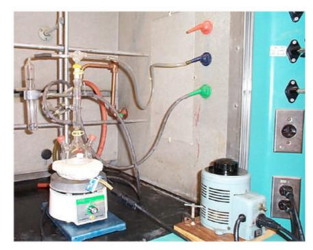
Fig. 2. Apparatus for benzoylation of dibenzyl tartrate.
