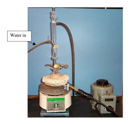
Fig. 1. Apparatus for esterification of tartaric acid.
