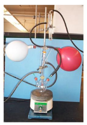
Fig. 3. Apparatus for hydrogenation.
