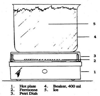
Figure 2: Apparatus for the Sublimation of Ferrocene
