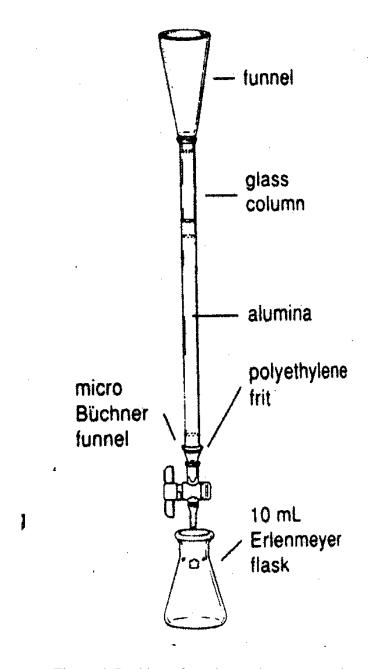
Figure 4. Packing of a column chromatography
