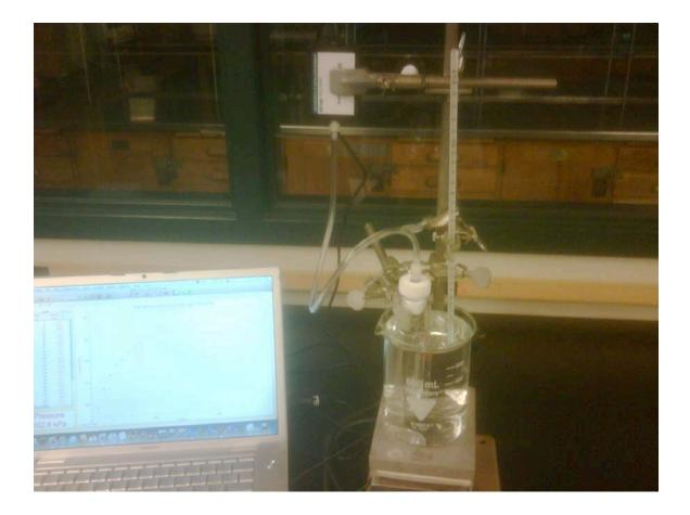
Figure 5. Apparatus for Measuring Kinetics of Catalase-H<sub>2</sub>O<sub>2</sub> Decomposition<sup>11</sup>
