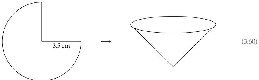
We could use many other shapes. However, a cone is easy to construct, and also falls without swishing back and forth (as a sheet of paper would) or flipping over (as long as you drop it point down).
