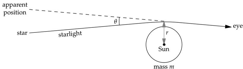
In Section 6.4.6, we used lumping to find that the gravitational field from a mass  $m$  bends light by an angle
