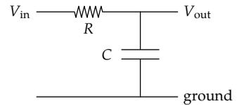
To help us make and use abstractions, let's imagine defocusing our eyes. Under blurry vision, the capacitor looks like a resistor that just happens to have a funny resistance  $R_C = 1/j\omega C$ . Now the entire circuit looks just like a pure-resistance circuit. Indeed, it is the simplest such circuit, a voltage divider. Its behavior is described by one number: the gain, which is the ratio of output to input voltage  $V_{\text{out}}/V_{\text{in}}$ .
