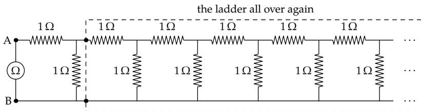
To find the resistance  $R$  across the ladder (in other words, what the ohmmeter measures between the nodes A and B), you represent the entire ladder as a single resistor  $R$ . Then the whole ladder is 1 ohm in series with the parallel combination of 1 ohm and  $R$ :
