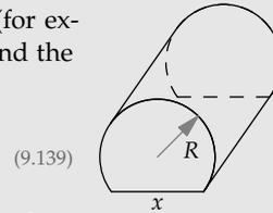
where  $x$  is the width of the contact strip. Then find the scaling exponent  $\gamma$  in  $F \propto \delta^\gamma$ , where  $F$  is the contact force and  $\delta$  is the tip compression. (In Problem 9.16, you computed the analogous scaling exponent for a sphere.)
