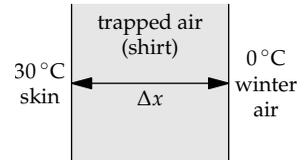
where  $\Delta T = T_2 - T_1$  is the temperature difference across a gap,  $\Delta x$  is the gap size, and  $K$  is the thermal conductivity of the gap material. Here, the gap material is air—the clothing serves to trap the air.
