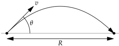
Now the problem contains four quantities:  $R$ ,  $v$ ,  $g$ , and  $\theta$ . Four quantities containing two independent dimensions (for example, L and T) produce two independent dimensionless groups. A reasonable pair is the launch angle  $\theta$ —which is already dimensionless—and, based on the proportional-reasoning result,  $Rg/v^2$ . Then the most general dimensionless statement is
