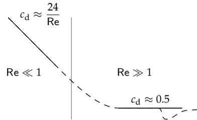
The dashed line interpolates between the extremes. The final twist is that at  $Re \sim 3 \times 10^5$ , the boundary layer becomes turbulent (Problem 7.23), and the drag coefficient drops significantly. With that caveat, we have explained the main features of drag, a ubiquitous force in the living world.
