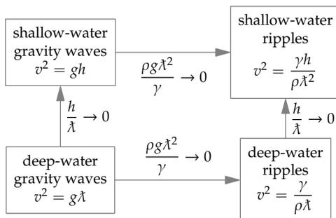
These waves are therefore ripples on shallow water. (They are hard to make, because ripples are tiny, smaller than a few millimeters, yet the water depth must be even smaller.)
