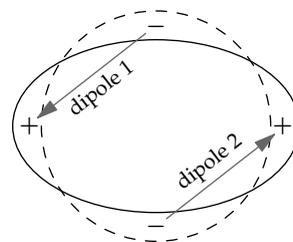
Just as the dipole field is the dimensionless derivative of the monopole field (Section 9.3.2), the quadrupole field is the dimensionless derivative of the dipole field. Thus, if the pulsating object has size  $l$ , so that the two dipoles are separated by a distance comparable to  $l$ , then at the boundary between the near and far fields (at  $r \sim c/\omega$ ), the fields are related by
