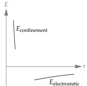
The slopes in the two regimes have opposite signs, so there is no smooth way to connect the two extreme segments without introducing a point where the slope is zero. This point, where the energy is a minimum, is nature's choice for the ground state of hydrogen.
