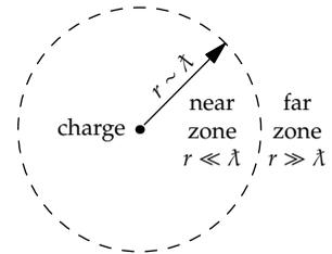
With  $\tilde{\lambda}$  as the comparison length, the dimensionless ratio determining whether  $r$  is small or large is  $r/\tilde{\lambda}$ , which is  $r\omega/c_s$ . At the boundary between the near and far zones,  $r \sim \tilde{\lambda}$ .
