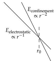
The stable middle regime is the one chosen by nature. Then  $r$ , the radius of hydrogen, is comparable to our special radius  $r_0$ . The special radius, and therefore  $r$ , is determined by equating electrostatic and confinement energies, which is how we found the Bohr radius  $a_0$  in Section 6.5.2. Thus, the radius of hydrogen is the Bohr radius and results from competition between electrostatics and quantum mechanics.
