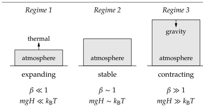
In the first regime, the atmosphere is expanding: The molecules have so much thermal energy that they escape farther from Earth. In the third regime, the atmosphere is contracting: The molecules do not have enough thermal energy to resist gravity as it pulls them back to Earth. The happy medium, where the atmosphere is stable, is the middle regime.
