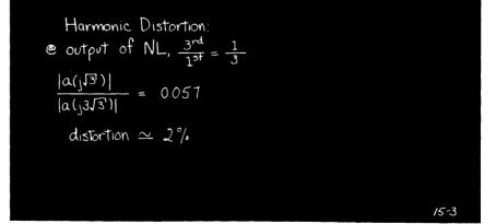
Describing-function analysis offers a way to apply the powerful frequency-domain methods that are so useful in linear-systems analysis to nonlinear systems. The describing function indicates the gain-and-phase shift that a nonlinear element provides to an input sinusoid, considering only the fundamental component of the output.
