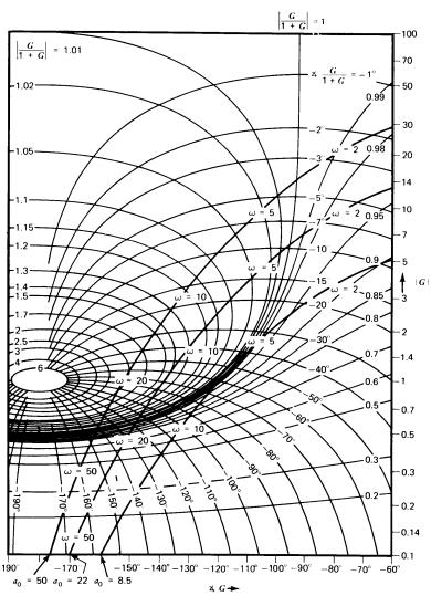
= 8.5  $a \rightarrow a$ Determination of closed-loop transfer function for  $a(s) = a_0 / [(s + 1)(0.1s + 1)]$ , f = 1.
