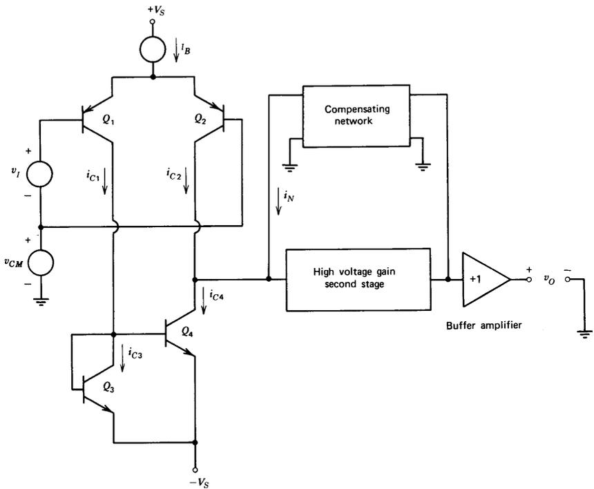
**Figure 13.43** Operational-amplifier model.
