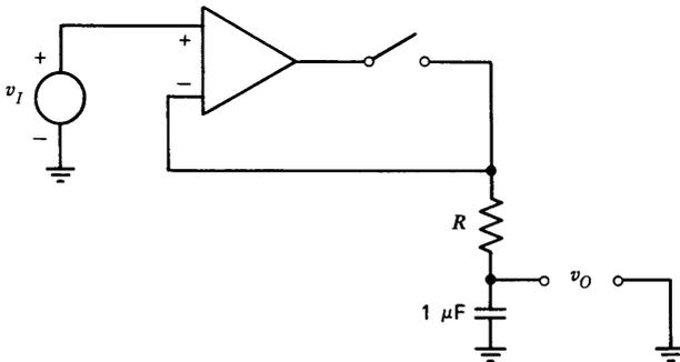
Figure 13.51 Sample-and-hold circuit.
