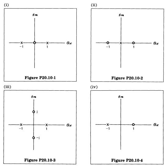
(d) Determine which, if any, of the pole-zero plots in part (c) could correspond to an odd time function. For those that could, indicate the required ROC.
