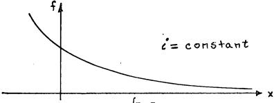
With the current constant, the drop in  $\int \tilde{H} \cdot d\bar{k}$  across the gap increases with x, and hence the field in the gap is reduced by increasing x.
