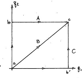
First carry out this line integral along the contour A: from  $a \rightarrow b$ ,  $q_1 = 0$ , while from  $b \rightarrow c$ ,  $dq_2 = 0$ . Hence,
