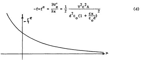
The energy converted to mechanical form is  $\int f^e dx$ . The contribution to this integral from d+c and b+a in the figure is zero. Hence,
