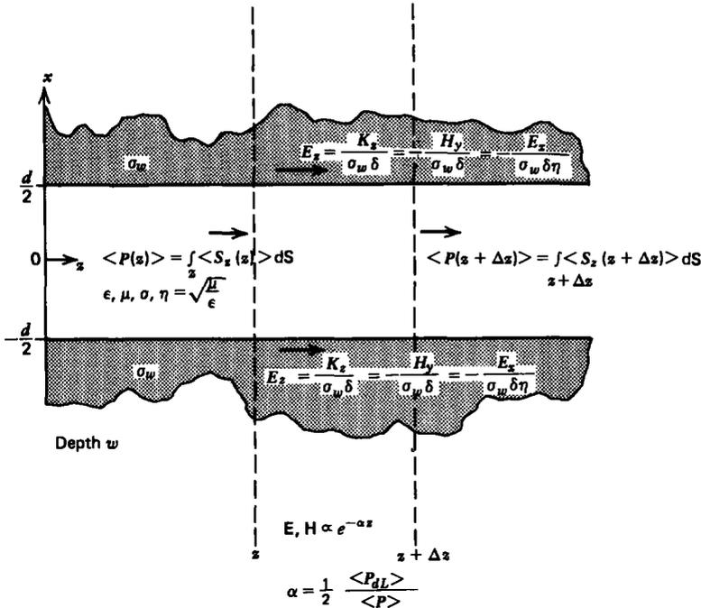
Figure 8-16 A transmission line with lossy walls and dielectric results in waves that decay as they propagate. The spatial decay rate  $\alpha$  of the fields is approximately proportional to the ratio of time average dissipated power per unit length  $\langle P_{dL} \rangle$  to the total time average electromagnetic power flow  $\langle P \rangle$  down the line.
