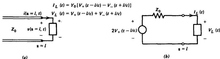
Figure 8-13 A transmission line with an (a) arbitrary load at the  $z=l$  end can be analyzed from the equivalent circuit in (b). Since  $V_+$  is known, calculation of the load current or voltage yields the reflected wave  $V_-$ .
