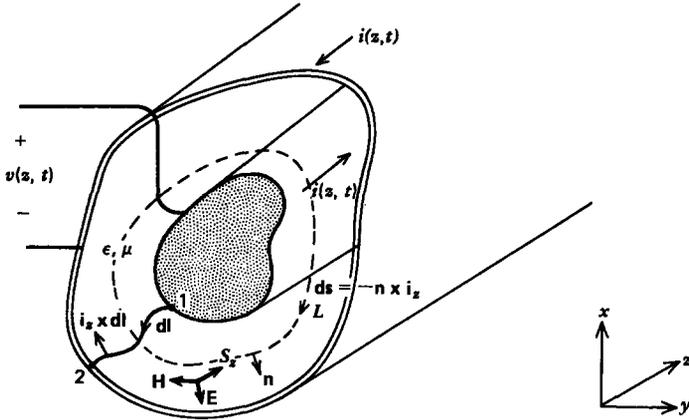
Figure 8-4 A general transmission line has two perfect conductors whose cross-sectional area does not change in the direction along its  $z$  axis, but whose shape in the transverse  $xy$  plane is arbitrary. The electric and magnetic fields are perpendicular, lie in the transverse  $xy$  plane, and have the same dependence on  $x$  and  $y$  as if the fields were static.
