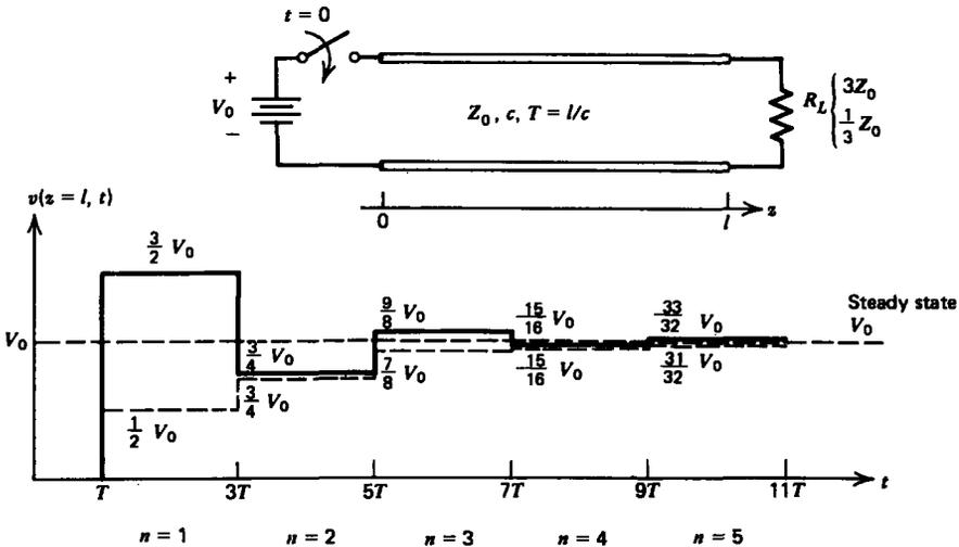
Figure 8-10 The load voltage as a function of time when  $R_s = 0$  and  $R_L = 3Z_0$  so that  $\Gamma_s \Gamma_L = -\frac{1}{2}$  (solid) and with  $R_L = \frac{1}{3}Z_0$  so that  $\Gamma_s \Gamma_L = \frac{1}{2}$  (dashed). The dc steady state is the same as if the transmission line were considered a pair of perfectly conducting wires in a circuit.
