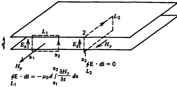
Figure 8-2 The potential difference measured between any two arbitrary points at different positions  $z_1$  and  $z_2$  on the transmission line is not unique—the line integral  $L_1$  of the electric field is nonzero since the contour has magnetic flux passing through it. If the contour  $L_2$  lies within a plane of constant  $z$  such as at  $z_3$ , no magnetic flux passes through it so that the voltage difference between the two electrodes at the same value of  $z$  is unique.
