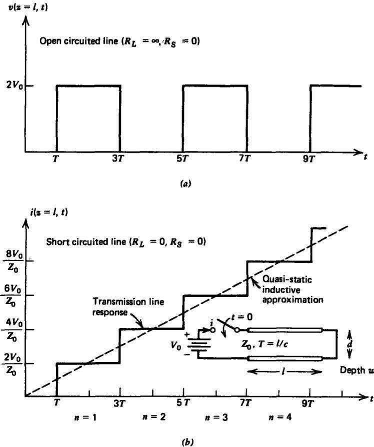
Figure 8-11 The (a) open circuit voltage and (b) short circuit current at the  $z = l$  end of the transmission line for  $R_L = 0$ . No dc steady state is reached because the system is lossless. If the short circuited transmission line is modeled as an inductor in the quasi-static limit, a step voltage input results in a linearly increasing current (shown dashed). The exact transmission line response is the solid staircase waveform.
