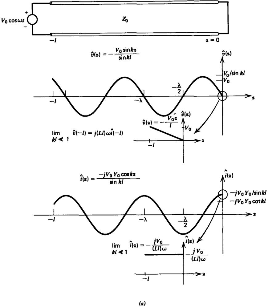
Figure 8-15 The voltage and current distributions on a (a) short circuited and (b) open circuited transmission line excited by sinusoidal voltage sources at  $z = -l$ . If the lines are much shorter than a wavelength, they act like reactive circuit elements. (c) As the frequency is raised, the impedance reflected back as a function of  $z$  can look capacitive or inductive making the transition through open or short circuits.
