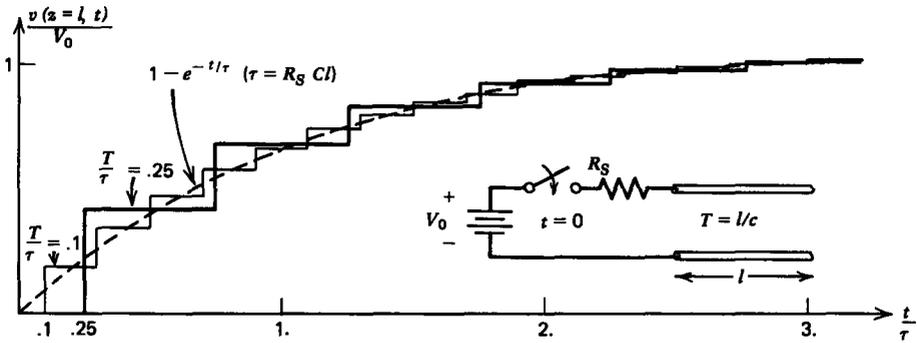
Figure 8-12 The open circuit voltage at  $z=l$  for a step voltage applied at  $t=0$  through a source resistance  $R_s$ , for various values of  $T/\tau$ , which is the ratio of propagation time  $T=l/c$  to quasi-static charging time  $\tau=R_s C l$ . The dashed curve shows the exponential rise obtained by a circuit analysis assuming the open circuited transmission line is a capacitor.
