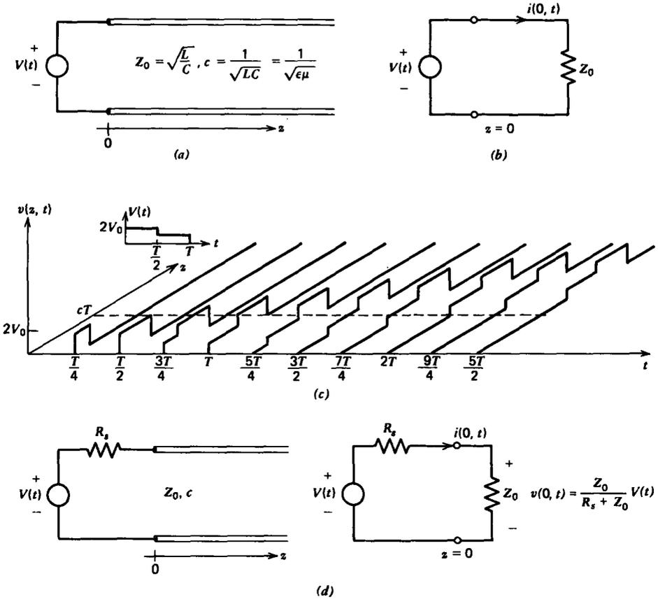
Figure 8-6 (a) A semi-infinite transmission line excited by a voltage source at  $z = 0$ . (b) To the source, the transmission line looks like a resistor  $Z_0$  equal to the characteristic impedance. (c) The spatial distribution of the voltage  $v(z, t)$  at various times for a staircase pulse of  $V(t)$ . (d) If the voltage source is applied to the transmission line through a series resistance  $R_s$ , the voltage across the line at  $z = 0$  is given by the voltage divider relation.
