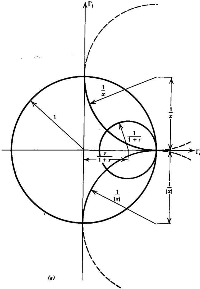
Figure 8-18 For passive loads the Smith chart is constructed within the unit circle in the complex  $\Gamma$  plane. (a) Circles of constant normalized resistance  $r$  and reactance  $x$  are constructed with the centers and radii shown. (b) Smith chart construction for various values of  $r$  and  $x$ .
