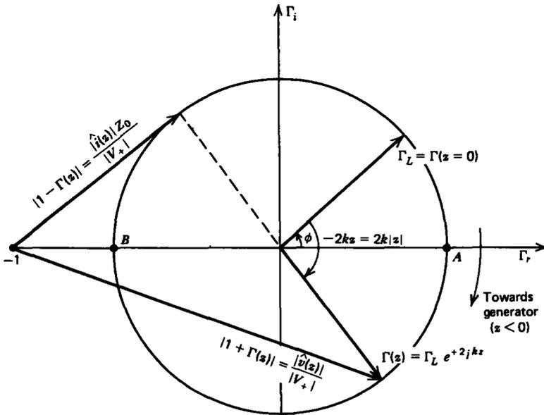
Figure 8-21 The voltage and current magnitudes along a transmission line are respectively proportional to the lengths of the vectors  $|1 + \Gamma(z)|$  and  $|1 - \Gamma(z)|$  in the complex  $\Gamma$  plane.
