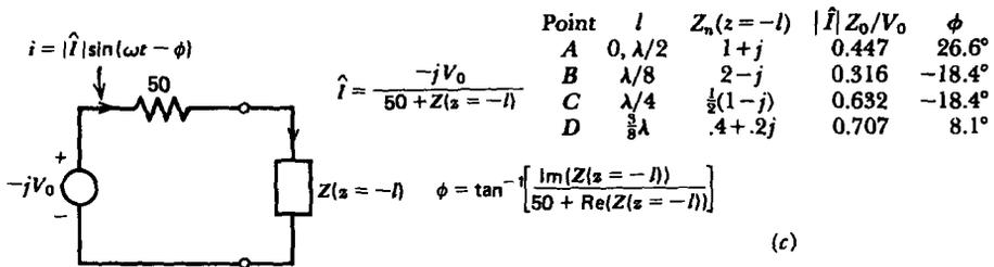
Figure 8-20 (a) The load impedance at  $z = 0$  reflected back to the source is found using the (b) Smith chart for various line lengths. Once this impedance is known the source current is found by solving the simple series circuit in (c).
