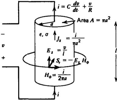
Figure 7-1 The power delivered to a lossy cylindrical capacitor  $vi$  is partly dissipated by the Ohmic conduction and partly stored in the electric field. This power can also be thought to flow in radially from the surrounding electric and magnetic fields via the Poynting vector  $\mathbf{S} = \mathbf{E} \times \mathbf{H}$ .
