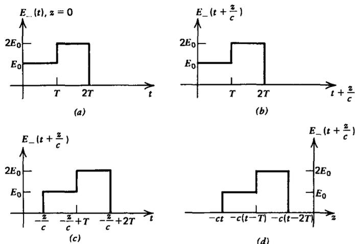
Figure 7-4 (a)  $E_-(t)$  at  $z = 0$  is a staircase pulse. (b)  $E_-(\phi)$  always has the same form of (a) when plotted versus  $\phi$ . Here  $\phi = t + z/c$ . (c) When plotted versus  $t$ , the pulse is translated in time where  $z$  must be negative to keep  $t$  positive. (d) When plotted versus  $z$ , it is translated but not inverted.
