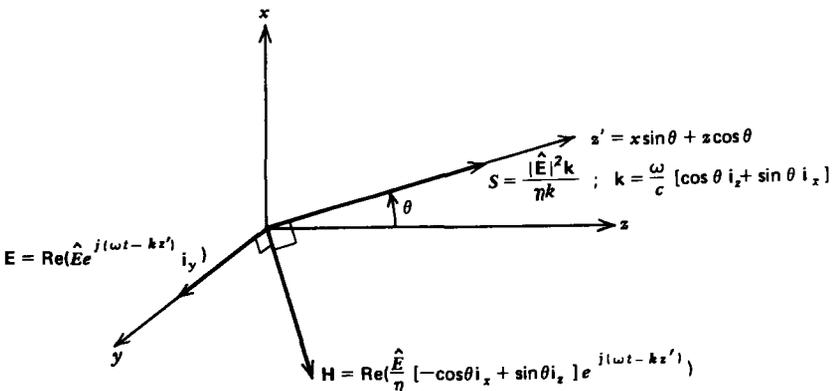
Figure 7-16 The spatial dependence of a uniform plane wave at an arbitrary angle  $\theta$  can be expressed in terms of a vector wavenumber  $\mathbf{k}$  as  $e^{-j\mathbf{k}\cdot\mathbf{r}}$ , where  $\mathbf{k}$  is in the direction of power flow and has magnitude  $\omega/c$ .
