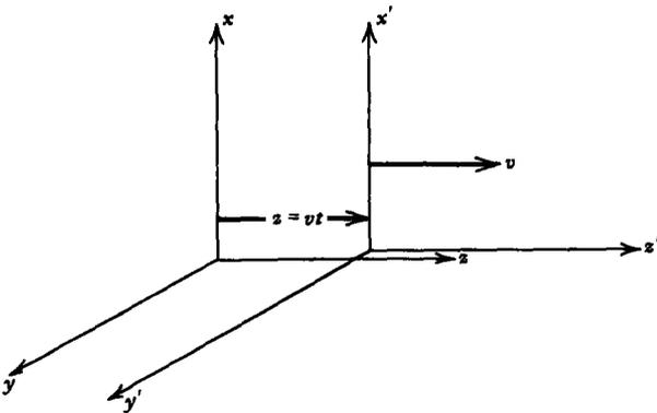
Figure 7-6 The primed coordinate system moves at constant velocity  $v\mathbf{i}_1$  with respect to a stationary coordinate system. The free space speed of an electromagnetic wave is  $c_0$  as measured by observers in either coordinate system no matter the velocity  $v$ .
