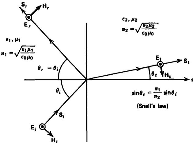
Figure 7-19 A summary of reflection and refraction phenomena across the interface separating two linear media. When  $\theta_i = \theta_B$  (Brewster's angle), there is no reflected ray. When  $\theta_i > \theta_c$  (critical angle), the transmitted fields decay with  $z$ .
