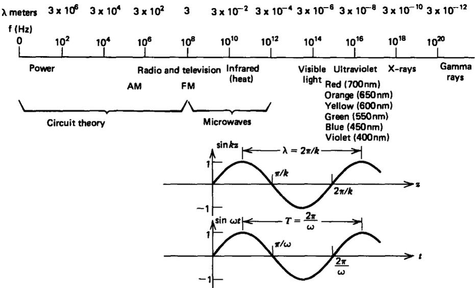
Figure 7-7 Time varying electromagnetic phenomena differ only in the scaling of time (frequency) and size (wavelength). In linear dielectric media the frequency and wavelength are related as  $f\lambda = c$  ( $\omega = kc$ ), where  $c = 1/\sqrt{\epsilon\mu}$  is the speed of light in the medium.
