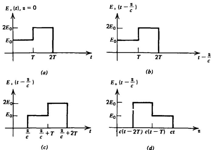
Figure 7-3 (a)  $E_+(t)$  at  $z = 0$  is a staircase pulse. (b)  $E_+(\phi)$  always has the same shape as (a) when plotted versus  $\phi$ , no matter what  $\phi$  is. Here  $\phi = t - z/c$ . (c) When plotted versus  $t$ , the pulse is translated in time where  $z$  must be positive to keep  $t$  positive. (d) When plotted versus  $z$ , it is translated and inverted. The pulse propagates at speed  $c$  in the positive  $z$  direction.
