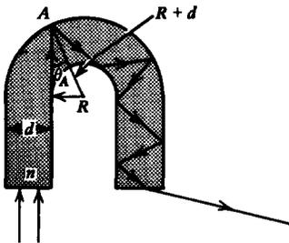
Figure 7-27 Light can be guided along a circularly bent fiber if  $R/d > 1/(n-1)$  as then there is always total internal reflection each time the light is incident on the walls.
