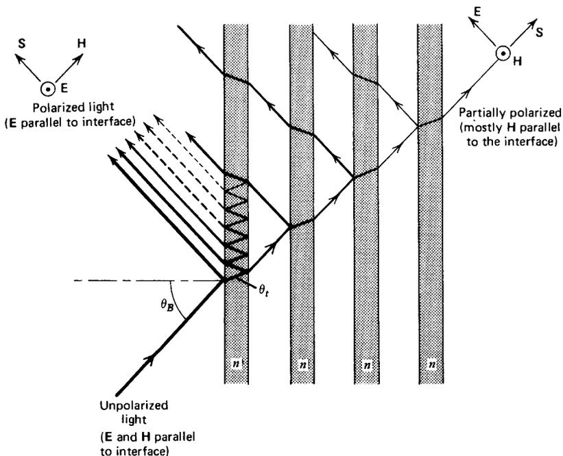
Figure 7-22 Unpolarized light incident upon glass with  $\mu = \mu_0$  can be polarized by reflection if it is incident at the Brewster's angle for the polarization with **H** parallel to the interface. The transmitted light becomes more polarized with **H** parallel to the interface by adding more parallel glass plates.
