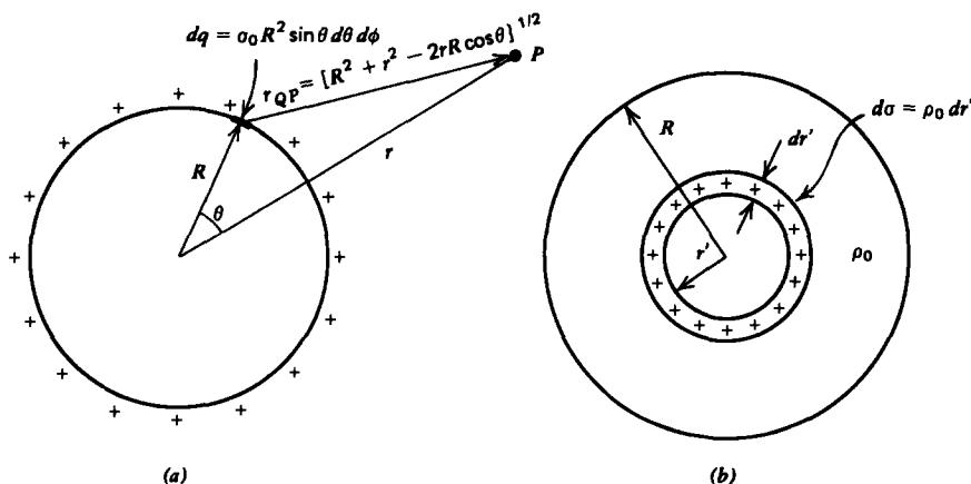
Figure 2-22 (a) A sphere of radius  $R$  supports a uniform distribution of surface charge  $\sigma_0$ . (b) The potential due to a uniformly volume charged sphere is found by summing the potentials due to differential sized shells.
