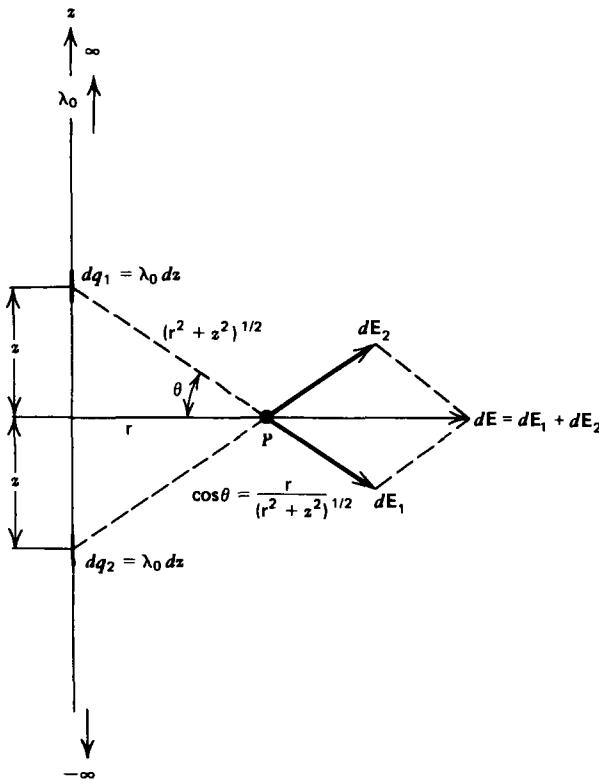
Figure 2-11 An infinitely long uniform distribution of line charge only has a radially directed electric field because the  $z$  components of the electric field are canceled out by symmetrically located incremental charge elements as also shown in Figure 2-8a.
