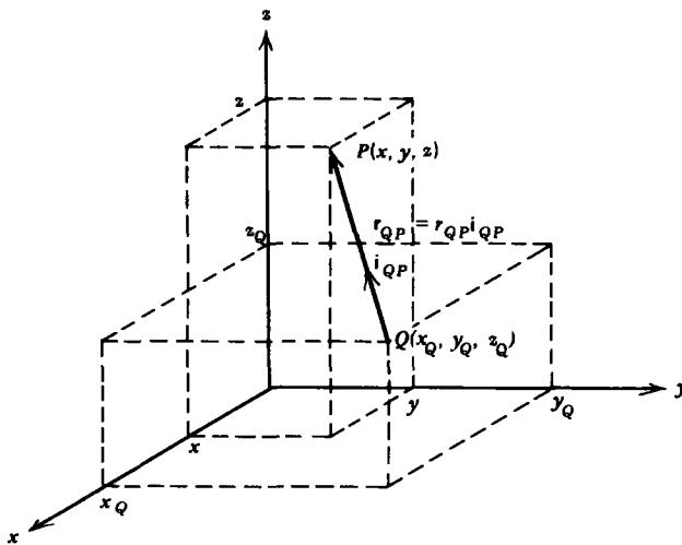
Figure 2-14 The vector distance  $r_{QP}$  between two points  $Q$  and  $P$ .
