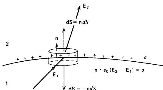
Figure 2-19 Gauss's law applied to a differential sized pill-box surface enclosing some surface charge shows that the normal component of  $\epsilon_0 \mathbf{E}$  is discontinuous in the surface charge density.
