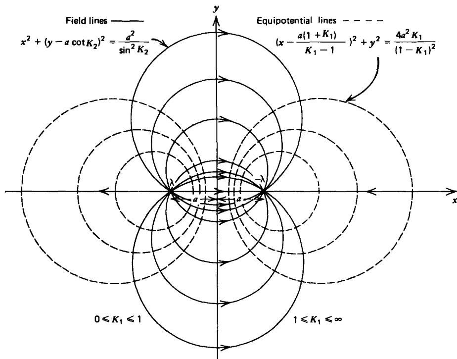
Figure 2-24 (a) Two parallel line charges of opposite polarity a distance  $2a$  apart. (b) The equipotential (dashed) and field (solid) lines form a set of orthogonal circles.
