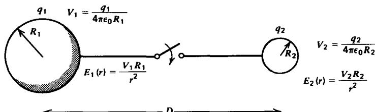
Figure 2-23 The charges on two spheres a long distance apart ( $D \gg R_1 + R_2$ ) must redistribute themselves when connected by a wire so that each sphere is at the same potential. The surface electric field is then larger at the smaller sphere.
