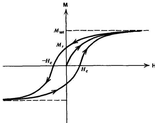
Figure 5-20 Ferromagnetic materials exhibit hysteresis where the magnetization saturates at high field strengths and retains a net remanent magnetization  $\mathbf{M}$ , even when  $\mathbf{H}$  is zero. A coercive field  $-H_c$  is required to bring the magnetization back to zero.
