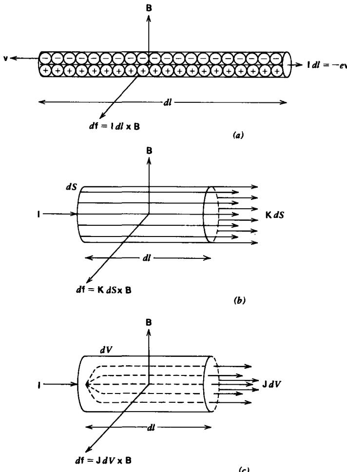
Figure 5-2 Moving line, surface, and volume charge distributions constitute currents. (a) In metallic wires the net charge is zero since there are equal amounts of negative and positive charges so that the Coulombic force is zero. Since the positive charge is essentially stationary, only the moving electrons contribute to the line current in the direction opposite to their motion. (b) Surface current. (c) Volume current.
