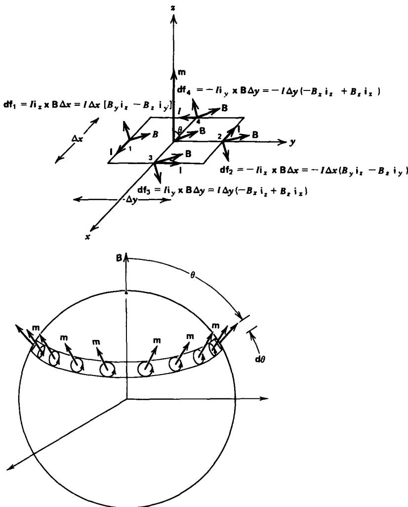
Figure 5-18 (a) A torque is exerted on a magnetic dipole with moment at an angle  $\theta$  to an applied magnetic field. (b) From Boltzmann statistics, thermal agitation opposes the alignment of magnetic dipoles. All the dipoles at an angle  $\theta$ , together have a net magnetization in the direction of the applied field.
