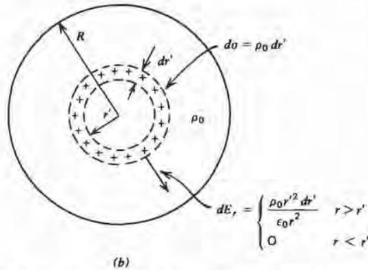
Figure 2-17 (a) Gaussian spheres for a uniformly charged sphere show that the electric field outside the sphere is again the same as if all the charge  $Q = \frac{4}{3}\pi R^3 \rho_0$  were concentrated as a point charge at  $r = 0$ . (b) The solution is also obtained by summing the contributions from incremental spherical shells of surface charge.
