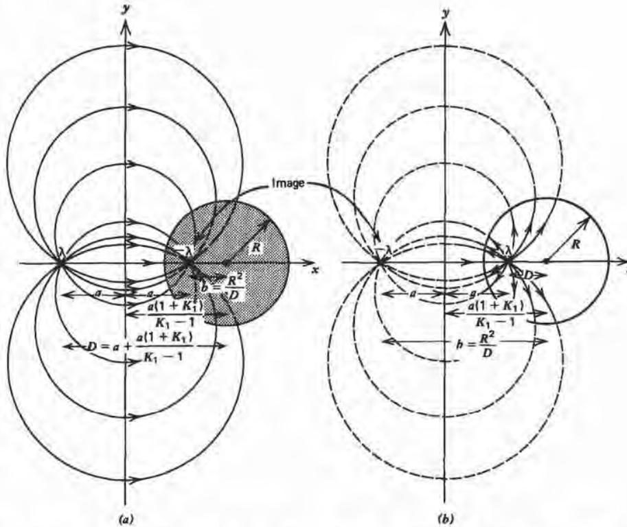
Figure 2-25 The electric field surrounding a line charge  $\lambda$  a distance  $D$  from the center of a conducting cylinder of radius  $R$  is the same as if the cylinder were replaced by an image charge  $-\lambda$ , a distance  $b = R^2/D$  from the center. (a) Line charge outside cylinder. (b) Line charge inside cylinder.
