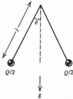
A total charge  $Q$  is deposited on the two balls of the electroscope. The angle  $\theta$  from the normal obeys a relation of the form
