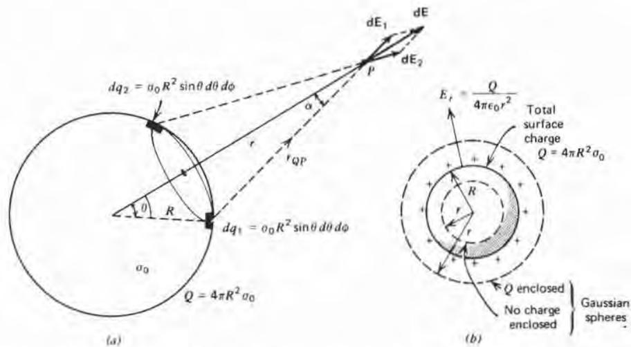
Figure 2-16 A sphere of radius  $R$  with uniformly distributed surface charge  $\sigma_0$ . (a) Symmetrically located charge elements show that the electric field is purely radial. (b) Gauss's law, applied to concentric spherical surfaces inside ( $r < R$ ) and outside ( $r > R$ ) the charged sphere, easily shows that the electric field within the sphere is zero and outside is the same as if all the charge  $Q = 4\pi R^2 \sigma_0$  were concentrated as a point charge at the origin.
