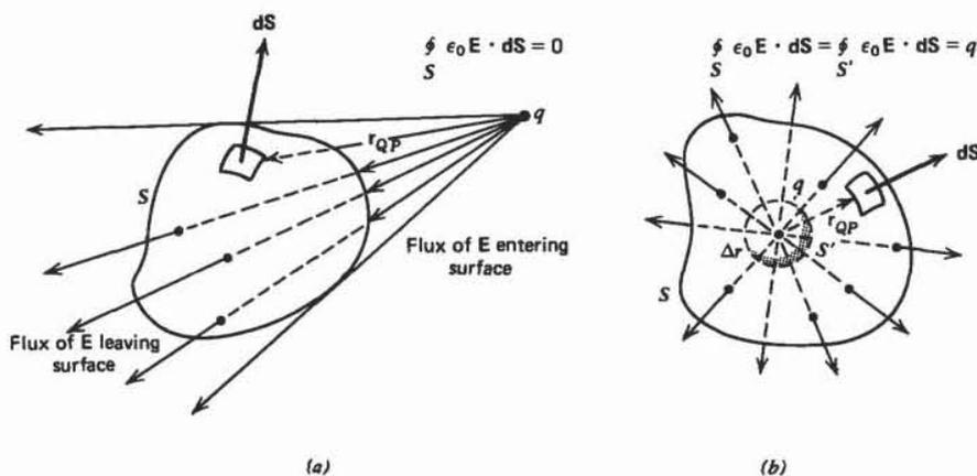
Figure 2-15 (a) The net flux of electric field through a closed surface  $S$  due to an outside point charge is zero because as much flux enters the near side of the surface as leaves on the far side. (b) All the flux of electric field emanating from an enclosed point charge passes through the surface.
