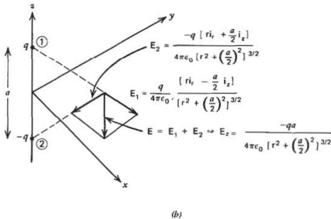
Figure 2-8 Two equal magnitude point charges are a distance  $a$  apart along the  $z$  axis. (a) When the charges are of the same polarity, the electric field due to each is radially directed away. In the  $z = 0$  symmetry plane, the net field component is radial. (b) When the charges are of opposite polarity, the electric field due to the negative charge is directed radially inwards. In the  $z = 0$  symmetry plane, the net field is now  $-z$  directed.
