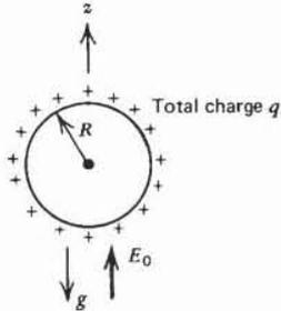
A spherical droplet of radius  $R$  and effective mass density  $\rho_m$  carries a total charge  $q$  in a gravity field  $g$ . What electric field  $E_0\mathbf{i}_z$  will suspend the charged droplet? Millikan found by this method that all droplets carried integer multiples of negative charge  $e = -1.6 \times 10^{-19}$  coul.
