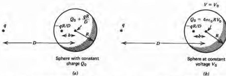
Figure 2-29 (a) If a conducting sphere carries a constant charge  $Q_0$  or (b) is at a constant voltage  $V_0$ , an additional image charge is needed at the sphere center when a charge  $q$  is nearby.
