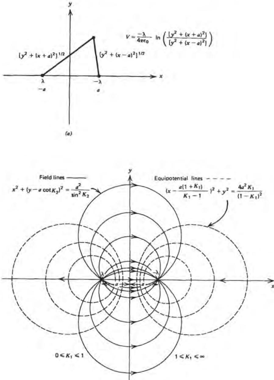
Figure 2-24 (a) Two parallel line charges of opposite polarity a distance  $2a$  apart. (b) The equipotential (dashed) and field (solid) lines form a set of orthogonal circles.
