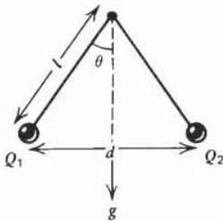
placed on the balls so that they are a distance  $d$  apart. A charge  $Q_1$  is placed on ball 1. What is the charge  $Q_2$  on ball 2?
