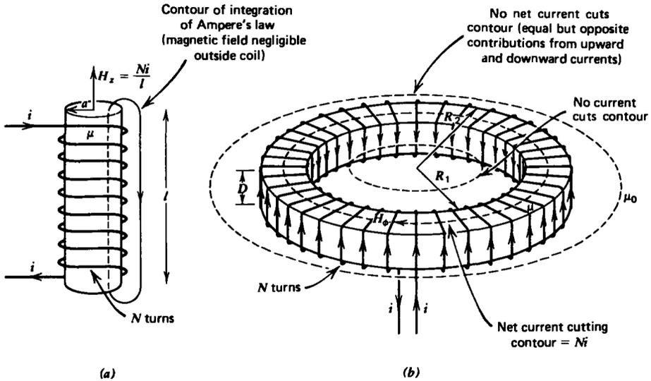
Figure 6-10 Inductances. (a) Solenoidal coil; (b) toroidal coil.
