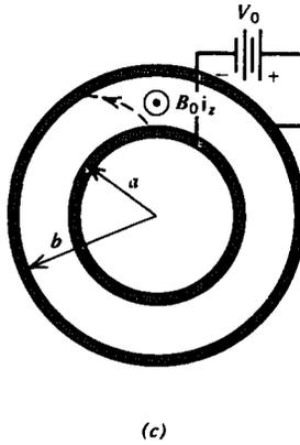
(c) A magnetron is built with coaxial electrodes where electrons are injected from  $r = a, \phi = 0$  with zero initial velocity. Using the relations from Table 1-2,
