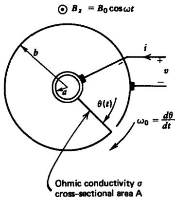
20. An MHD machine is placed within a magnetic circuit.
