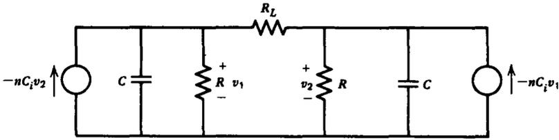
(b) If  $n = 10$ ,  $C_i = 2$  pf, and  $C = 10$  pf with  $R_L = R$ , what is the minimum value of  $R$  for self-excitation?
