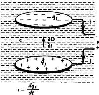
Figure 3-19 The conduction current  $i$  that travels through the connecting wire to an electrode in a lossless capacitor is transmitted through the dielectric medium to the opposite electrode via displacement current. No charge carriers travel through the lossless dielectric.
