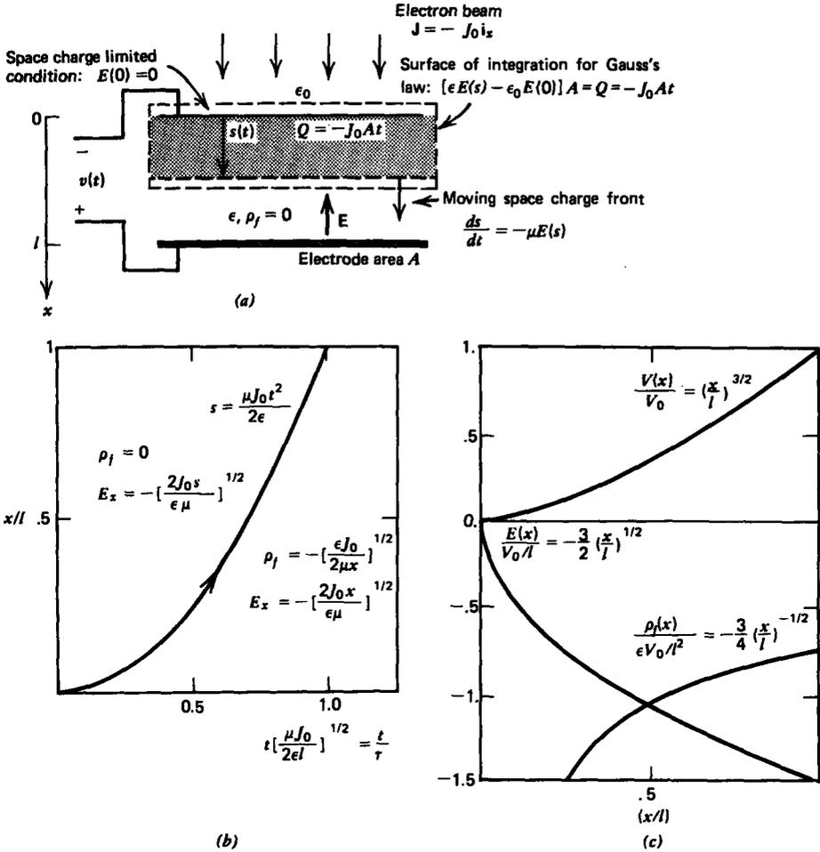
Figure 3-27 (a) An electron beam carrying a current  $-J_0 \mathbf{i}_x$  is turned on at  $t = 0$ . The electrons travel through the dielectric with mobility  $\mu$ . (b) The space charge front, at a distance  $s$  in front of the space charge limited interface at  $x = 0$ , travels towards the opposite electrode. (c) After the transit time  $t_c = [2\epsilon l/\mu J_0]^{1/2}$  the steady-state potential, electric field, and space charge distributions.
