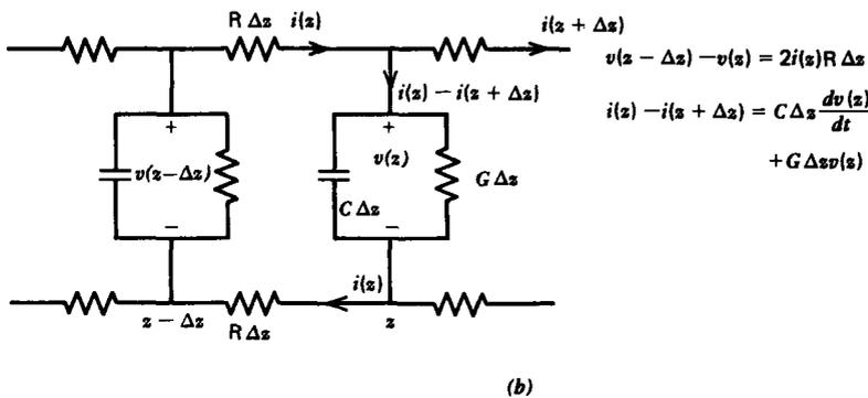
Figure 3-23 Lossy parallel plate electrodes with finite Ohmic conductivity  $\sigma_c$  enclose a lossy dielectric with permittivity  $\epsilon$  and conductivity  $\sigma$ . (a) This system can be modeled by a distributed resistor-capacitor network. (b) Kirchoff's voltage and current laws applied to a section of length  $\Delta z$  allow us to describe the system by partial differential equations.
