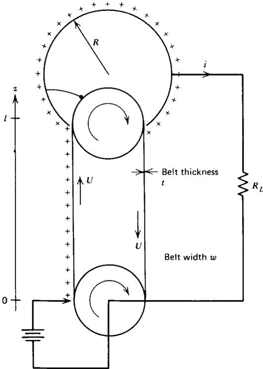
58. A Van de Graaff generator has a lossy belt with Ohmic conductivity  $\sigma$  traveling at constant speed  $U$ . The charging point at  $z = 0$  maintains a constant volume charge density  $\rho_0$  on the belt at  $z = 0$ . The dome is loaded by a resistor  $R_L$  to ground.
