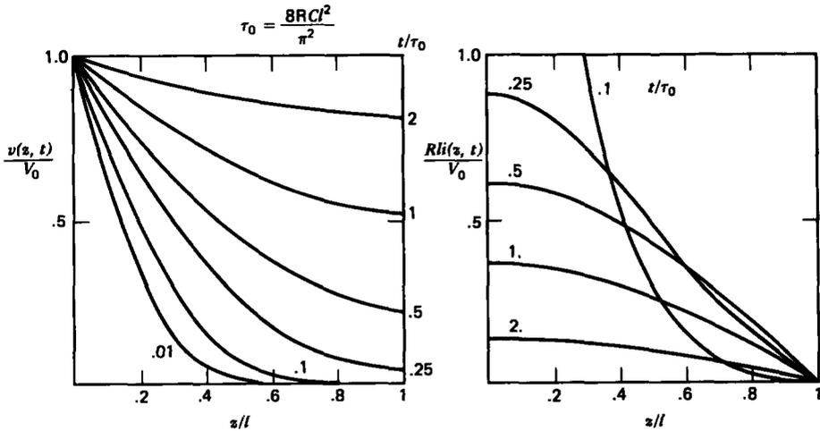
Figure 3-24 The transient voltage and current spatial distributions for various times for the lossy line in Figure 3-23a with  $G = 0$  for a step voltage excitation at  $z = 0$  with the  $z = l$  end open circuited. The diffusion effects arise because of the lossy electrodes where the longest time constant is  $\tau_0 = 8RCl^2/\pi^2$ .
