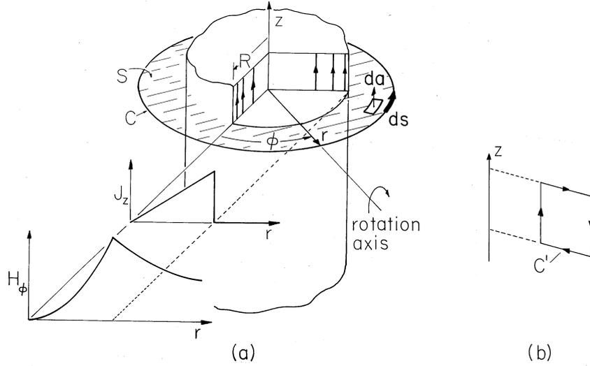
**Fig. 1.4.2** Axially symmetric current distribution and associated radial distribution of azimuthal magnetic field intensity. Contour  $C$  is used to determine azimuthal  $\mathbf{H}$ , while  $C'$  is used to show that the  $z$ -directed field must be uniform.
