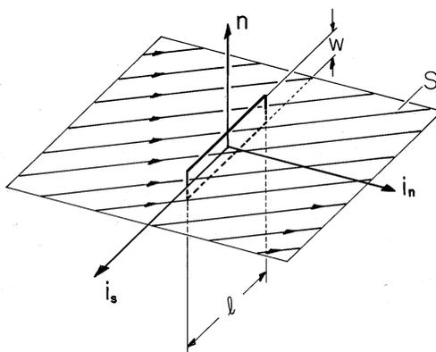
**Fig. 1.4.7** Ampère's integral law is applied to surface  $S'$  enclosed by a rectangular contour that intersects a surface  $S$  carrying the current density  $\mathbf{K}$ . In terms of the unit normal to  $S$ ,  $\mathbf{n}$ , the resulting continuity condition is given by (16).
