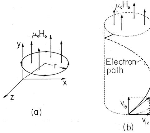
**Fig. 1.1.3** (a) In a uniform magnetic flux density  $\mu_o\mathbf{H}_o$  and with no initial velocity in the  $y$  direction, an electron has a circular orbit. (b) With an initial velocity in the  $y$  direction, the orbit is helical.
