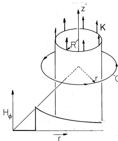
**Fig. 1.4.6** Uniform current density  $K_o$  is  $z$  directed in circular cylindrical shell at  $r = R$ . Radially discontinuous azimuthal field shown is determined using the contour at arbitrary radius  $r$ .
