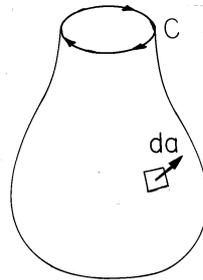
**Fig. 1.5.1** Contour  $C$  enclosing an open surface can be thought of as the drawstring of a bag that can be closed to create a closed surface.
