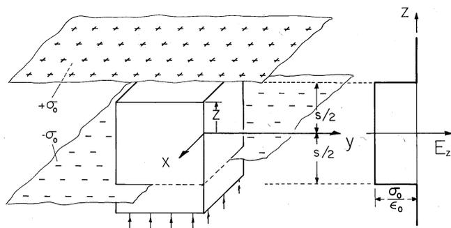
**Fig. 1.3.8** Sheets of surface charge and volume of integration with upper surface at arbitrary position  $x$ . With field  $E_o$  due to external charges equal to zero, the distribution of electric field is the discontinuous function shown at right.
