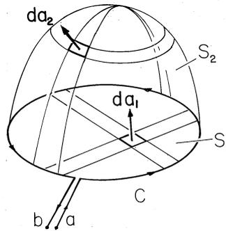
**Fig. 1.7.1** Contour  $C$  follows loop of wire having terminals  $a - b$ . Because each has the same enclosing contour, the net magnetic flux through surfaces  $S_1$  and  $S_2$  must be the same.
