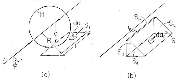
**Fig. 1.7.2** (a) The field of a line current induces a flux in a horizontal rectangular coil. (b) The open surface has the coil as an enclosing contour. Rather than being in the plane of the contour, this surface is composed of the five segments shown.
