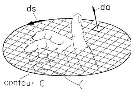
**Fig. 1.4.1** Surface  $S$  is enclosed by contour  $C$  having positive direction determined by the right-hand rule. With the fingers in the direction of  $ds$ , the thumb passes through the surface in the direction of positive  $da$ .
