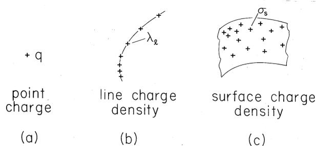
**Fig. 1.3.3** Singular charge distributions: (a) point charge, (b) line charge, (c) surface charge.
