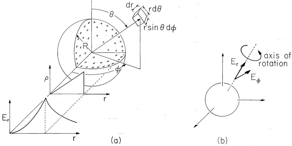
**Fig. 1.3.2** (a) Spherically symmetric charge distribution, showing radial dependence of charge density and associated radial electric field intensity. (b) Axis of rotation for demonstration that the components of  $\mathbf{E}$  transverse to the radial coordinate are zero.
