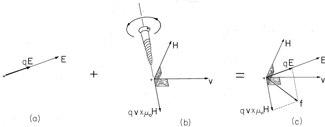
**Fig. 1.1.1** Lorentz force  $\mathbf{f}$  in geometric relation to the electric and magnetic field intensities,  $\mathbf{E}$  and  $\mathbf{H}$ , and the charge velocity  $\mathbf{v}$ : (a) electric force, (b) magnetic force, and (c) total force.
