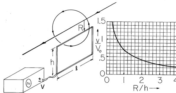
**Fig. 1.6.4** Demonstration of voltmeter reading induced at terminals of a coil in accordance with Faraday's law. To plot data on graph, normalize voltage to  $V_0$  as defined with (11). Because  $I$  is the peak current,  $v$  is the peak voltage.
