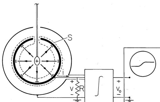
**Fig. 1.5.5** When a charge  $q$  is introduced into an essentially grounded metal sphere, a charge  $-q$  is induced on its inner surface. The integral form of charge conservation, applied to the surface  $S$ , shows that  $i = dq/dt$ . The net excursion of the integrated signal is then a direct measurement of  $q$ .
