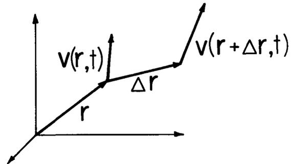
Fig. 7.14.1. Positions in the flow separated by an incremental distance  $\Delta \vec{r}$ .
