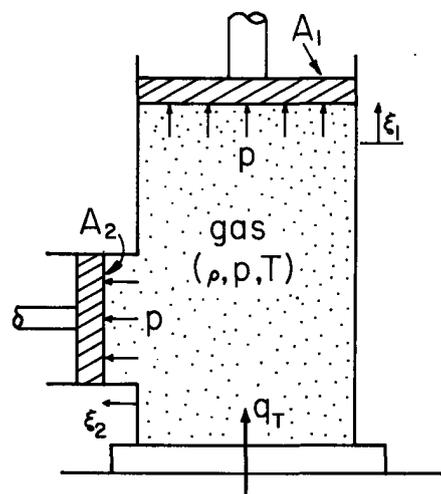
Fig. 7.22.1. Schematic view of lumped-parameter thermodynamic subsystem.
