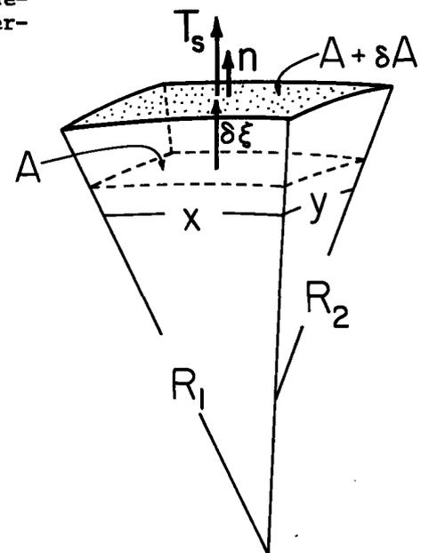
Fig. 7.6.1. Section of interface that suffers perpendicular displacement  $\delta\xi$  to make new surface  $\delta A$ .
