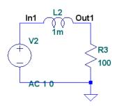
The impedance of the resistor is  $Z_R = R$  (constant for all frequencies) and the impedance of the inductor is  $Z_L = i\omega L$ .
