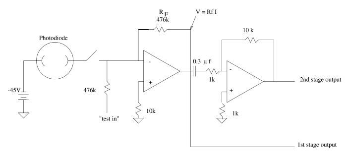
FIG. 7: Diagram of the photo-diode and preamplifier circuit.
