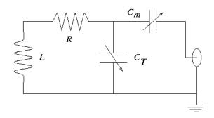
FIG. 9: Schematatic diagram of NMR probe circuit. The connector on the right goes off to the source and any detection circuitry.
