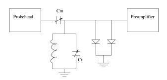
FIG. 5: Schematic of the probehead circuit.
