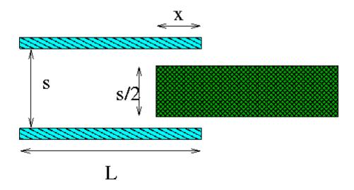
Two flat square metal plates with sides of length *L* are arranged parallel to each other with a separation of *S* where  $S \le L$ . This assumption allows you to neglect the fringing effects due to the finite size of the plates. A charge +Q is moved from the top plate to the bottom. A third, uncharged, conducting plate of the same size with thickness  $\frac{S}{2}$  is slid between the other two to a
