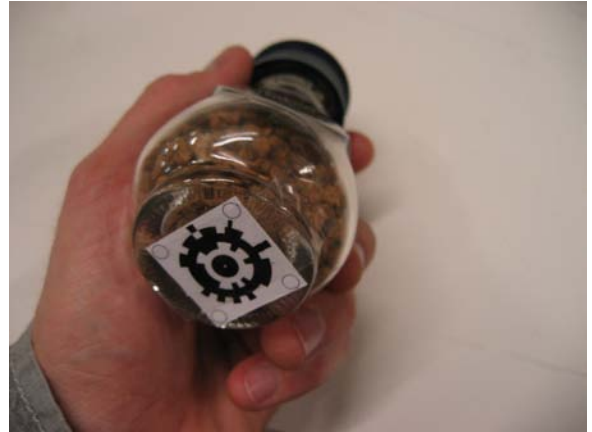
Tag placed on the bottom of the object to be read by the scanning surface.
