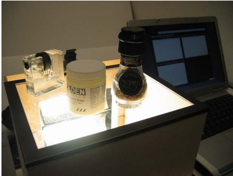
Three objects placed on the scanning surface of the Object Investigator system.
