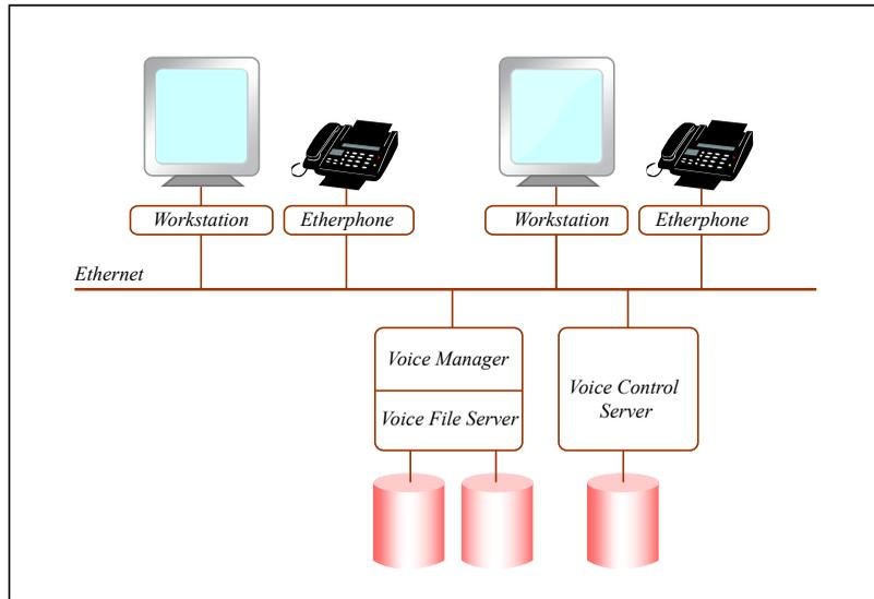
**Figure 11.1.** Etherphone architecture. (Figure by MIT OpenCourseWare, after Terry and Swinehart, 1988.)
