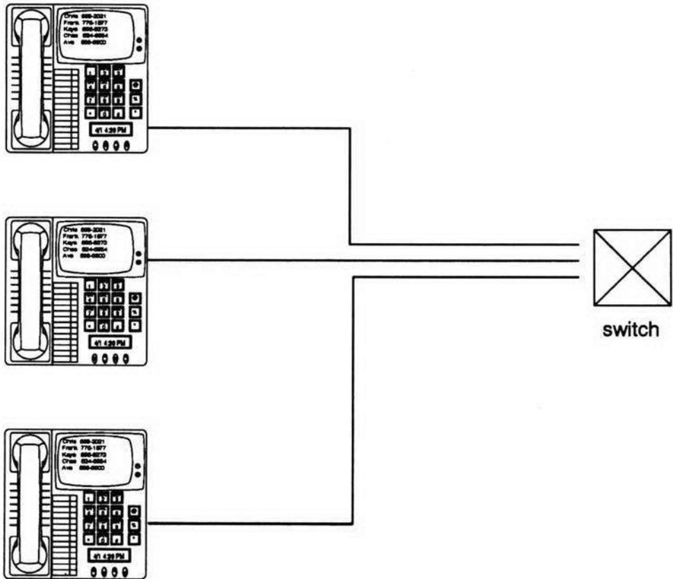
**Figure 11.9.** A distributed architecture of enhanced telephones.
