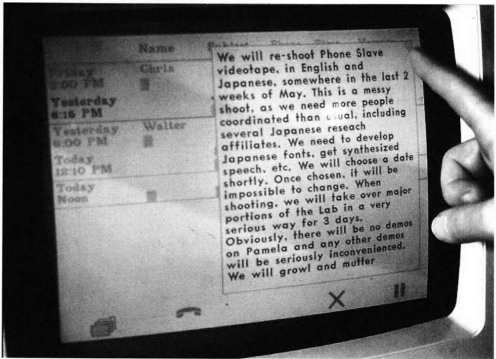
**Figure 11.12.** Phone Slave used a pop-up window to display a text message. From Schmandt and Arons, "Phone Slave: A Graphical Telecommunications System." Reprinted with permission from the 1984 *SID International Symposium Digest of Technical Papers*, edited by Jay Morreale. Vol. 25, New York: Palisades Institute for Research Services, Inc. June, 1984. pp. 146–149.
