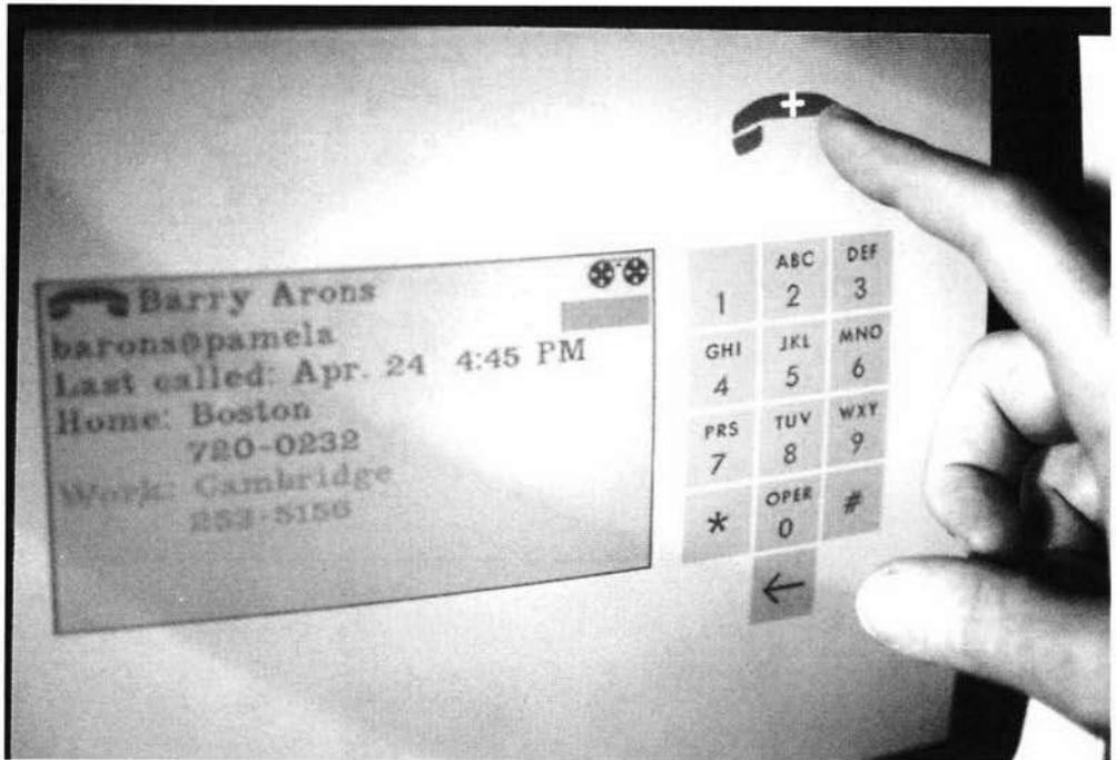
**Figure 11.14.** Phone Slave's telephone dialing view. From Schmandt and Arons, "Phone Slave: A Graphical Telecommunications System." Reprinted with permission from the *1984 SID International Symposium Digest of Technical Papers*, edited by Jay Morreale. Vol. 25, New York: Palisades Institute for Research Services, Inc. June, 1984. pp. 146-149.
