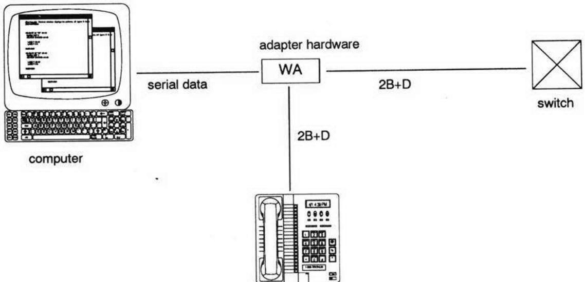
**Figure 11.4.** Architecture of the PX project. A workstation adapter, WA, allows a computer to interface to both the telephone instrument and the telephone switch by converting digital signalling protocols.
