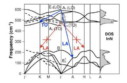
Fig. 3. Phonon energy as a function of phonon momentum and density of states (DOS) for InN redrawn from [12] in which  $E_{\rm LO} > 2E_{\rm LA}$  such that  $\rm LO \rightarrow 2LA$  (Klemens mechanism) is forbidden, whereas the  $\rm LO \rightarrow TO+LA$  (Ridley mechanism) can occur, although it is normally less likely and involves smaller loss of energy [13].
