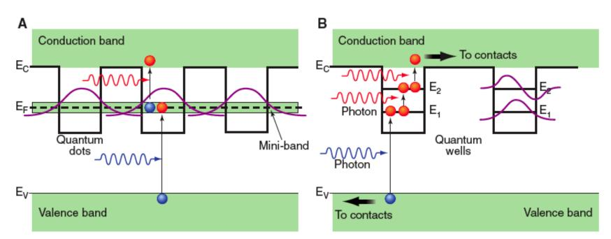
**Fig. 2.** Possible methods of circumventing the 31% efficiency limit for thermalized carriers in a single-band gap absorption threshold solar quantum conversion system. (**A**) Intermediate-band solar cell; (**B**) quantum-well solar cell. [Adapted from (2)]
