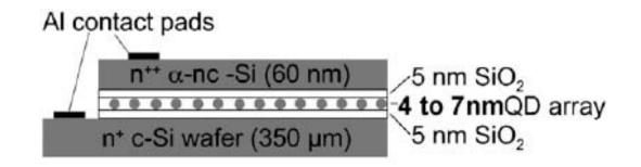
Fig. 3. Sample structure for SEC experiments.
