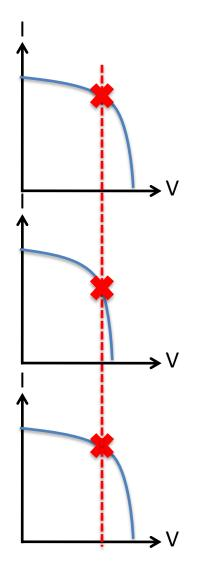
Cells in **Parallel** in a Module are matched in voltage.
