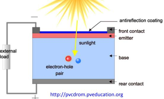
(2) Charge Separation: An electric field engineered into the material (pn junction) sweeps out electrons.
