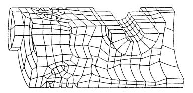
Figure 1.15: A cell decomposition (finite element mesh).
