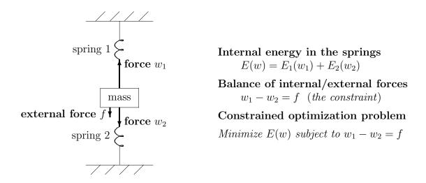
Figure 7.2: Minimum spring energy E(w) subject to balance of forces.
