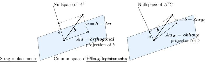
Figure 7.1: Ordinary and weighted least squares: min  $||b - Au||^2$  and  $||Wb - WAu||^2$ .
