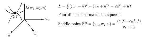
Figure 7.4:  $(w_1-u)^2$  and  $(w_2+u)^2$  go up,  $-2u^2$  goes down from the saddle point SP.
