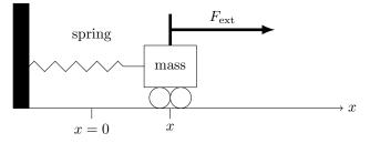
We set up the coordinate system so that at x = 0 the spring is relaxed, which means that it is exerting no force. This is called the **equilibrium position**.
