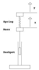
Figure 1. Spring-driven system
