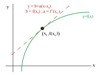
Figure 1: Tangent as a linear approximation to a curve
