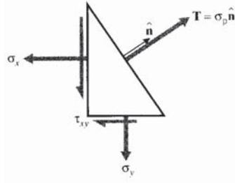
Figure 11: Traction vector normal to principal plane.
