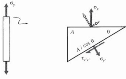
Figure 2: An inclined plane in a tensile specimen.
