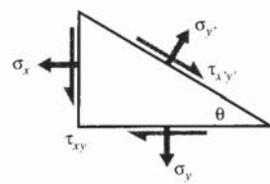
Figure 4: Stresses on inclined plane.
